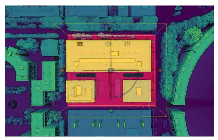
Inside cude highlighting of a point cloud (LiDAR HD, Montpellier, France)
