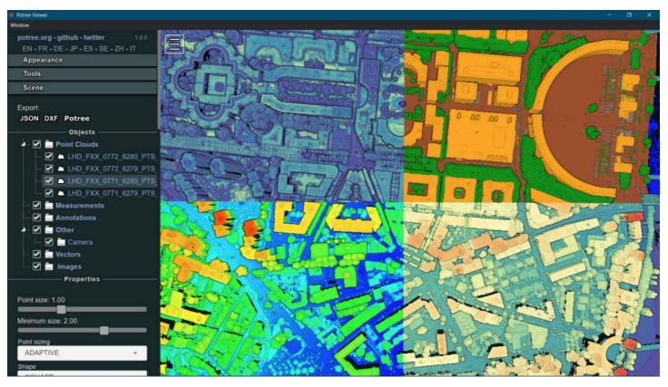
4 separated point clouds rendered with different styles (Intensity, classification, and elevation)
