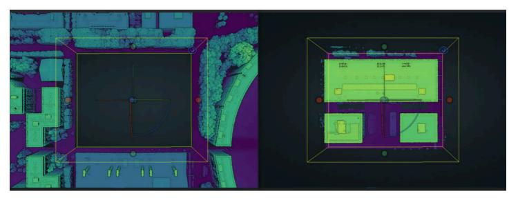
Clipping results, outside (left) and inside (right), (point cloud of LiDAR HD, Montpellier, France)
