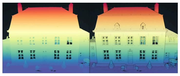
Same point cloud without EDL (left) and with it (right), Radius and Strenght parameters impact the degree of edge shadowing @ULB
