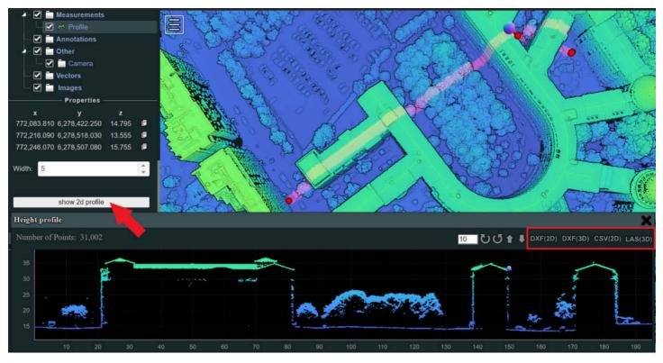
Profile extraction (point cloud of LiDAR HD, Montpellier, France)
